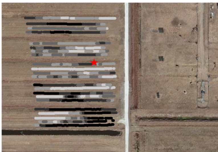
Fig. 36. Veris MSP3 mapping of EC, where increasing EC relates to increasingly darker colors. Relative EC index of 5.5 was measured at the forage points (red star symbols).
