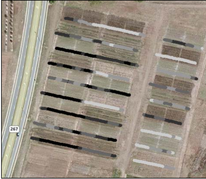
Fig. 24. Front office block (FOB) soil EC mapping. Electrical conductivity color gradient ranged from light gray (lowest values) to black (highest values). This is an indirect measure of soil nutrient content and it can also be associated with soil moisture, to some extent. Darker shades should be somewhat more fertile and perhaps finer textured that hold more moisture.
