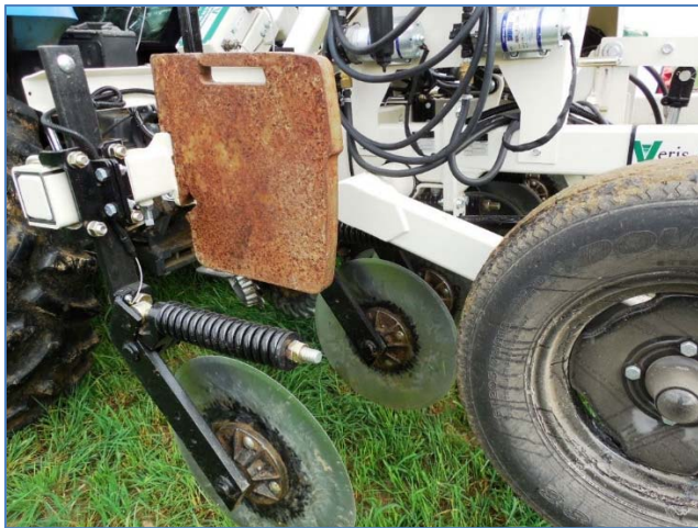
Fig. 2. Each coulter is fitted with an EC sensor to measure EC at two depth ranges (0 to 1 ft and 0 to 3 ft) simultaneously.
