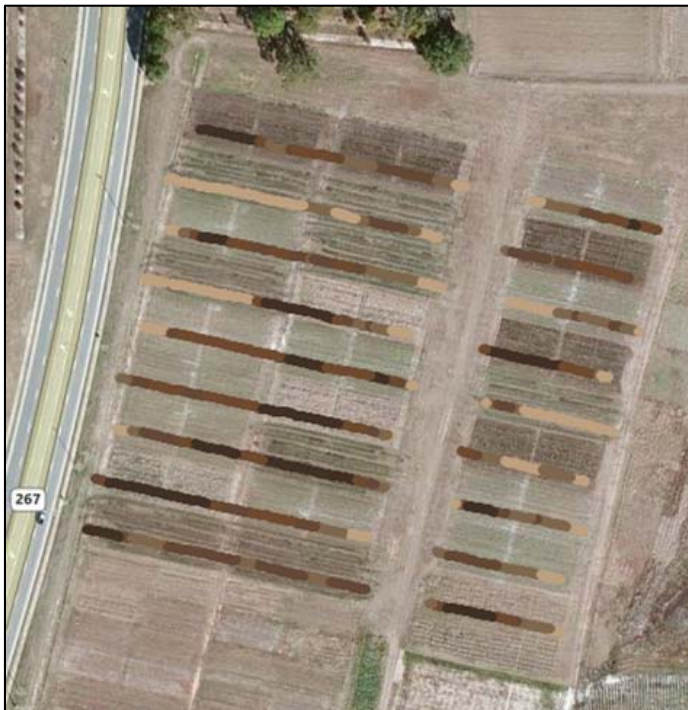
Fig. 26. Front office block (FOB) soil infrared (IR) mapping, which is related to soil organic matter (SOM). The IR color gradient ranged from beige (lowest SOM) to dark brown (highest SOM). This is an indirect measure of SOM. Darker shades should be somewhat more fertile and perhaps hold more moisture.
