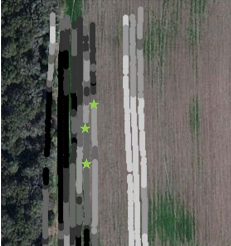
Fig. 31. Veris MSP3 mapping of EC, where increasing EC relates to increasingly darker colors. Relative EC index of 8.5 was measured at the forage points (star symbols).
