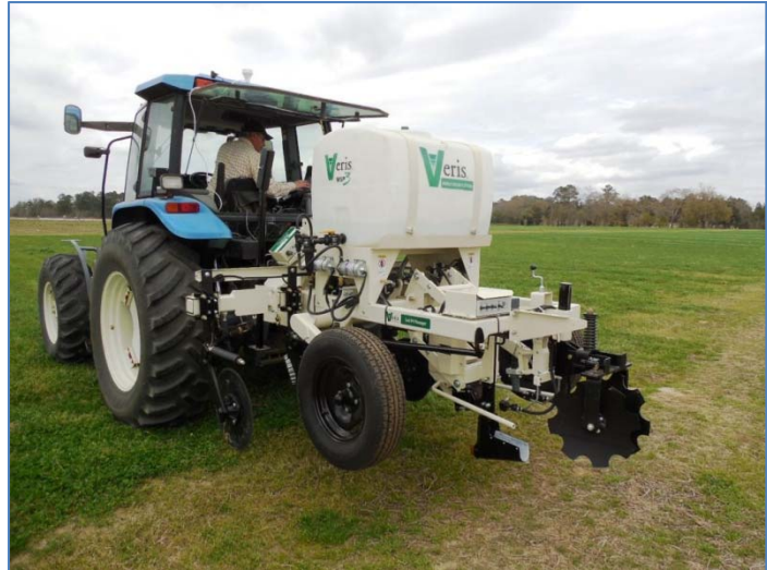
Fig. 1. Veris MSP3 prepared to map bahiagrass field.
