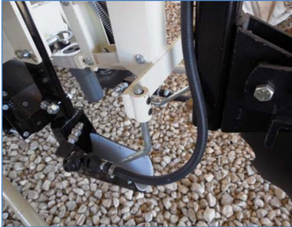
Fig. 4. After the soil sample is collected, the sensor (gray probe above cup) and cup meet, where the pH reading is taken. Following the reading, spray nozzles wash the sensor clean prior to the next sample collection.
