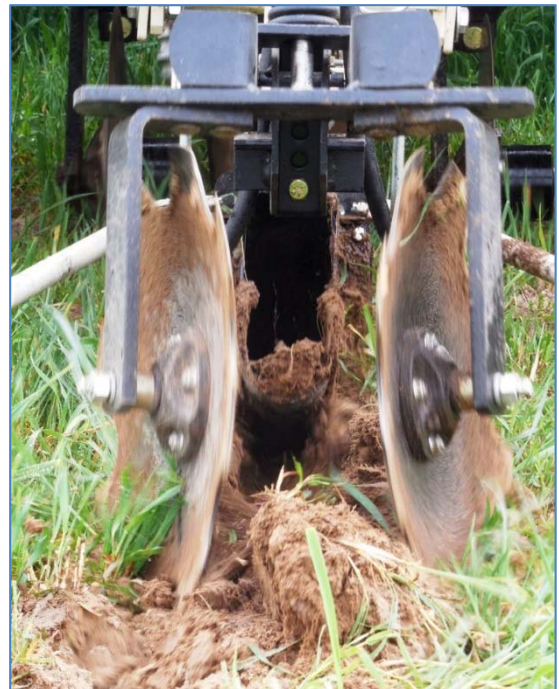
Fig. 3 Between two coulters (located behind the EC coulters), the pH sampling scoop prepares to collect soil sample for pH measurement.
