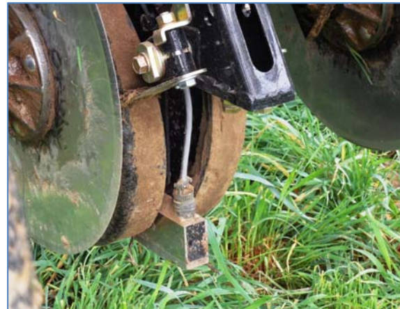
Fig. 5. In front of the pH sampler (close to tractor cab), lies the OM sensor (rectangular block). A sapphire window measures soil reflectance from IR and red light beams aimed at the soil.
