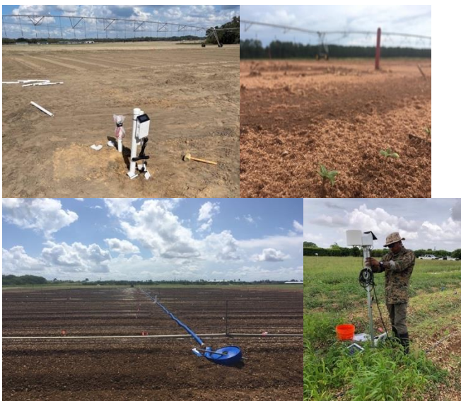
Figure 1. Field preparation across sites. Upper left: Lysimeter installation PSREU. Upper right: Irrigation installation and seedling emergence WFREC. Bottom: Irrigation (left) and soil moisture sensor (right) installation at TREC.
