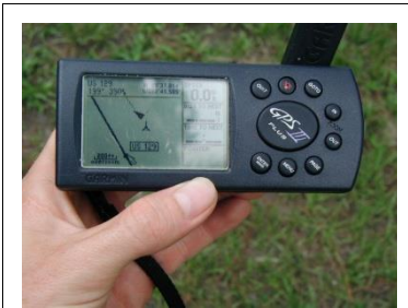
A simple Global Positioning System (GPS) unit. Foresters use GPS units to map forests and to pinpoint special locations accurately.
