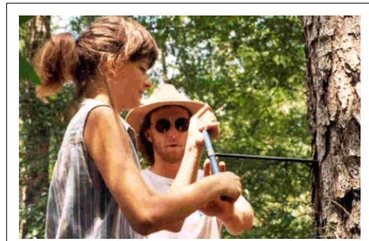
A student uses an increment borer at a summer camp at Withlacoochee State Forest.
